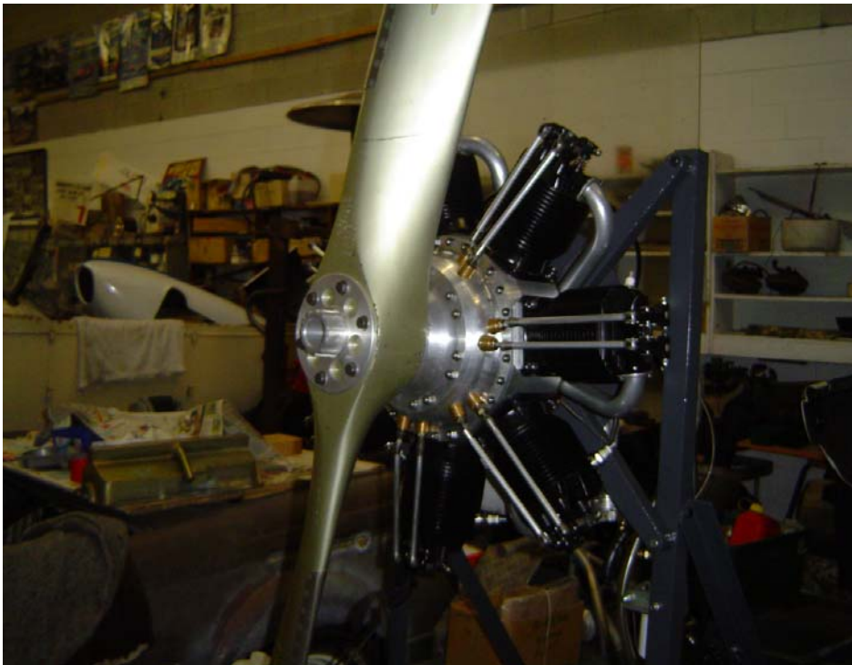
The Ralph Watson Rotary engine comprising of 7 cylinders which was started by Ralph and completed by Allan
